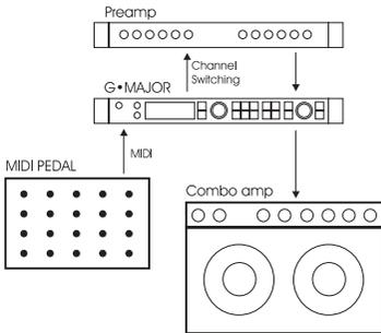
Using the return on the Combo's effect loop will in most cases give you a setup similar to the power-amp setup described above. Using the regular Input on the Combo gives you a "double-preamp" setup where you can use the tone controls on the Combo to color your sound. This introduces more noise than when using the Effect Return connection, but has become a popular setup with amplifiers like Vox AC 30, Fender Bassman etc.
