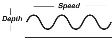
The basic illustration shows that the Chorus effect consists of both the original and the pitch modulated signal.
